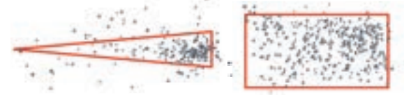
UNTREATED CRYGENICALLY TREATED Irregular and uneven shot pattern. Denser and more uniform shot pattern.
