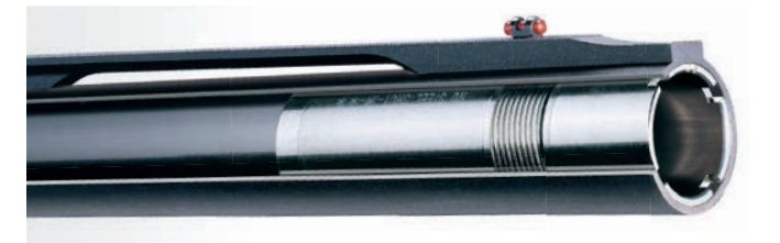
The Crio® System combines a barrel frozen to -300° F with a specially designed longer choke tube that is also cryogenically treated. The result is a denser, more uniform shot pattern that puts more pellets on target.
